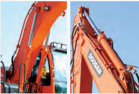
Heavy-duty boom, arm & cylinders
